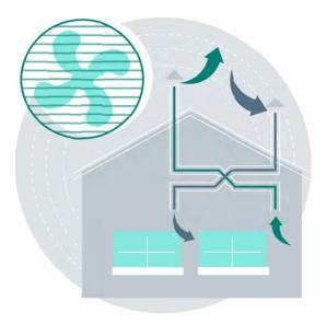
Ventilation must be designed to achieve 6–8 air changes per hour (ie the number of times per hour that the whole volume of air in each room is replaced by fresh air) in general areas. Fresh air is preferable to recirculated air. Flows less than six air changes per hour are inadequate to help prevent airborne microbial transmission.<sup>1</sup>
