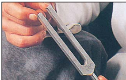
Figure 4. Aluminium tuning fork. Is best struck lightly as shown. Aluminium will hold a tune for much longer than the equivalent steel fork
