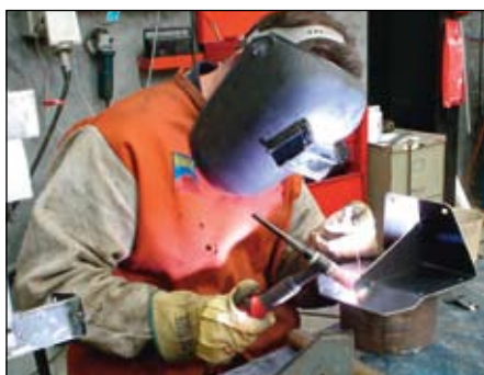
Figure 6. A safer GTA welding practice. This welder should also have protection to the back of the neck as well some fume extraction system in place. Reproduced with permission: Prototype Engineering Centre, 2006
