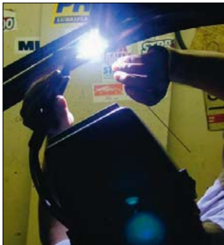
Figure 5. An example of unsafe welding practice. Note the bare hands and forearms. The welder is working close to the arc and his neck is also unsafely exposed
